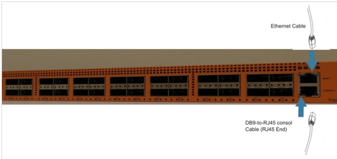
Figure 8: Connecting the Console and Management Ports
