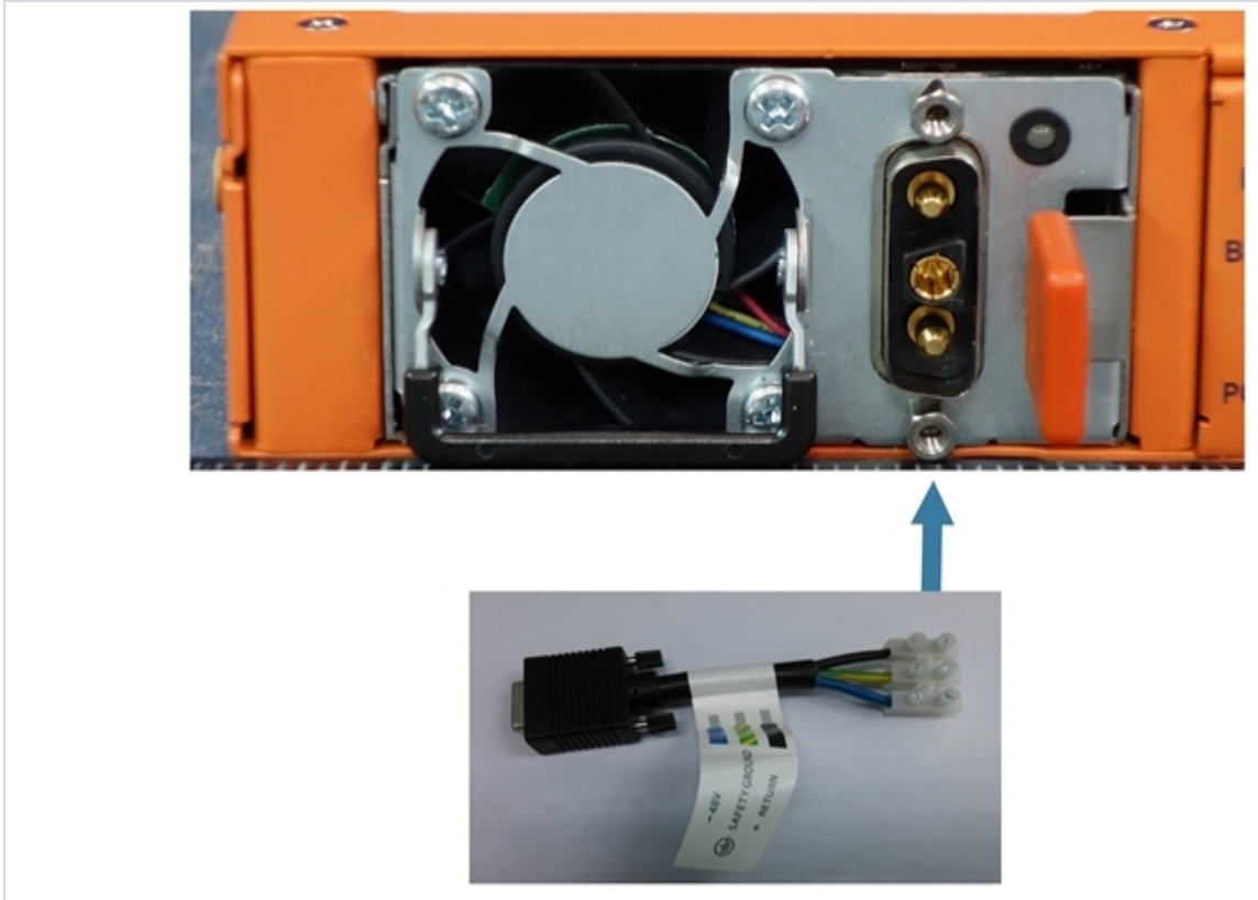
Figure 6: Connecting -48V DC Power Cable Adapter
