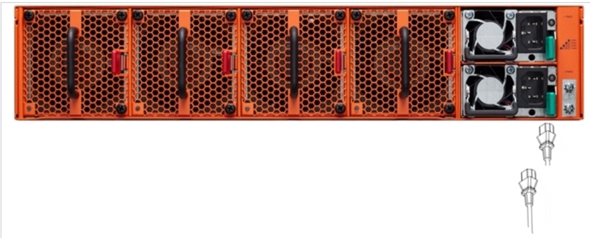
Figure 5: Connecting AC Power on a GigaVUE-TA200
