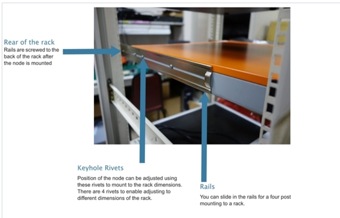
Figure 2: GigaVUE Traffic Aggregator with Rail Mounting for Four-Post Racks
